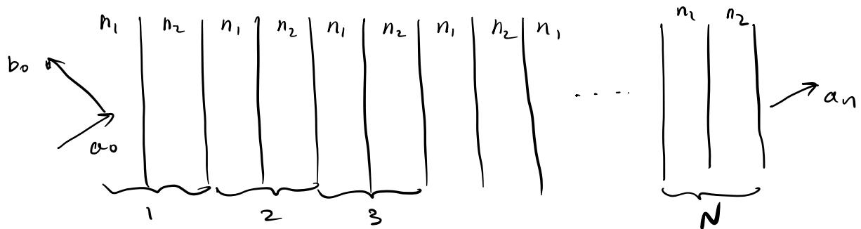
$$\text{reflection coefficient: } r_N = \frac{b_0}{a_0}$$
