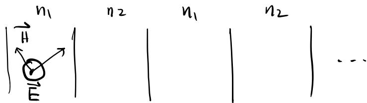
B.C.  $E_x$  and  $H_y$  are continuous at interfaces  $z = (n-1)\Lambda$  and  $z = n\Lambda - a$ .
