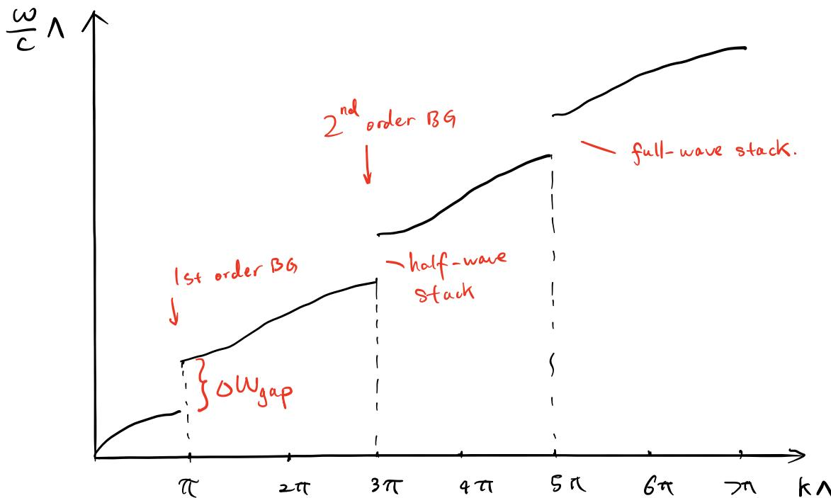
( Parameters :  $n_1 = 1.45$ ,  $n_2 = 2.65$ ,  $a = \frac{\lambda_0}{4n_1} = 259 \text{ nm}$ ,  $b = \frac{\lambda_0}{4n_2} = 142 \text{ nm}$ ,  $\lambda_0 = 1.5 \mu\text{m}$  )
