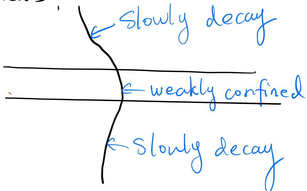
when d is small, wave is weakly guided in the waveguide.
