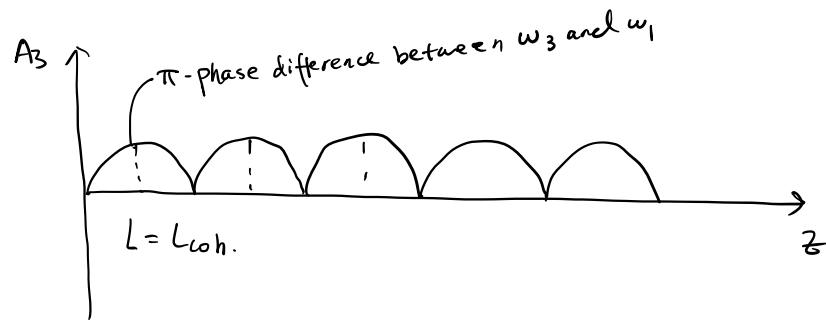
At  $L = L_{coh}$ , there's a  $\pi$  phase difference between  $w_3$  and  $w_1$ . By introducing QPM, we flip the sign of  $\text{d}e/\text{d}z$  at  $L_{coh}$ . Then  $\pi$  phase is regarded "o-phase" for  $w_3$  and  $w_1$ , at the next cycle.
