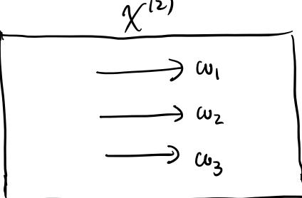
$$\left\{ \begin{array}{l} \frac{dA_3}{dt} = \frac{2i \text{deff} \omega_3^2}{k_3 c^2} A_1 A_2 e^{i\Delta k z} \\ \frac{dA_1}{dz} = \frac{2i \text{deff} \omega_1^2}{k_1 c^2} A_3 A_2^* e^{-i\Delta k z} \\ \frac{dA_2}{dz} = \frac{2i \text{deff} \omega_2^2}{k_2 c^2} A_3 A_1^* e^{-i\Delta k z} \end{array} \right. \quad \begin{array}{l} \text{①} \\ \text{②} \\ \text{③} \end{array}$$
