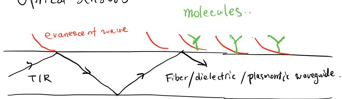
The absorbance of chemical/bio/gas molecules will interact with the evanescent field, and perturb the transmitted optical signal.
