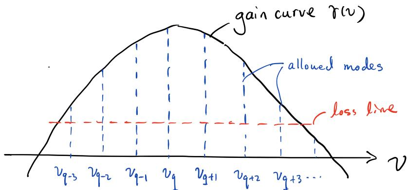
$$\text{Mode spacing: } v_q - v_{q-1} = \text{FSR} = \frac{c}{2nL}$$
