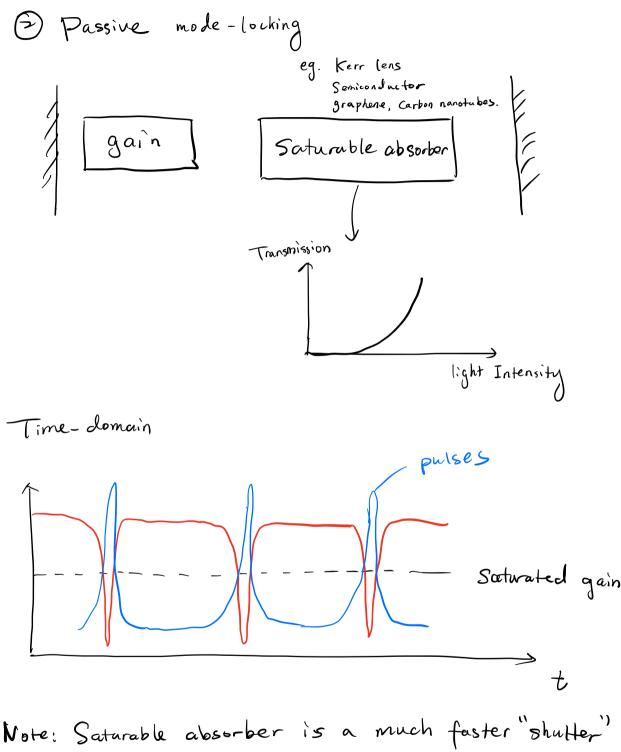
compared to external RF modulation. It allows for the generation of shorter pulses.
