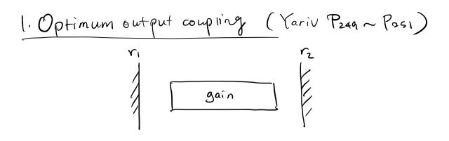
threshold condition. gain = loss.
