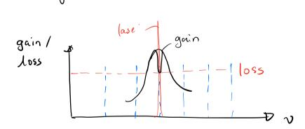
2 Make the reflector narrow band! gain/ 1055
