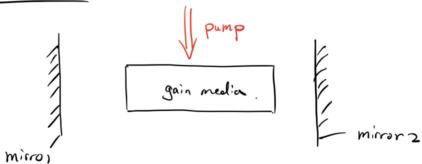
Three elements: ① gain medium, ② pump. ③ cavity.
