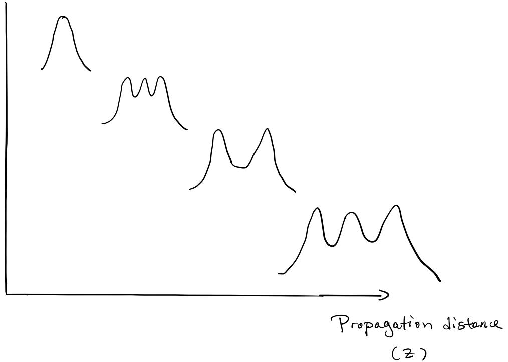
3. In case of unchirped input pulses, SPM always leads to spectral broadening. With linearly chirped input, pulse, spectral narrowing can occur!
